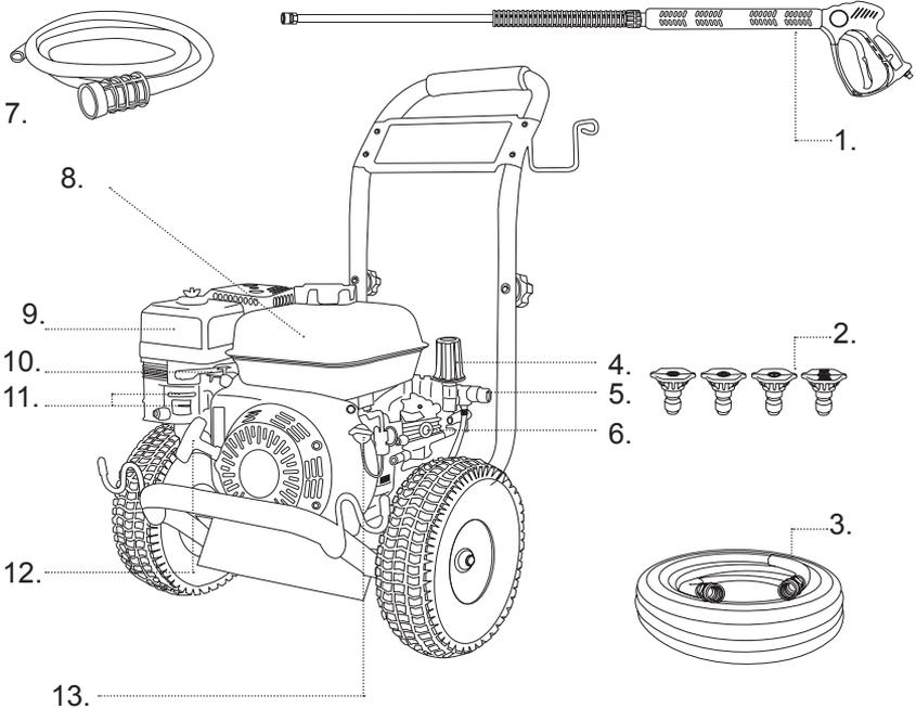
1. **Spray Gun** Controls the application of water onto cleaning surface with trigger device. Includes trigger lock. Allows you to switch between various spray tips.
