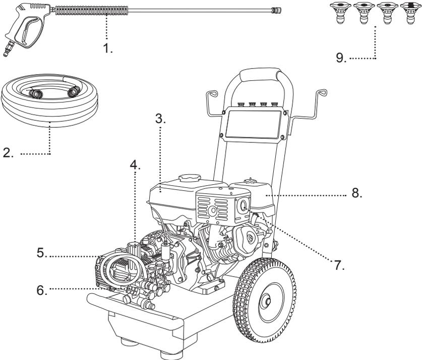
1. **Spray Gun** - Controls the application of water onto cleaning surface with trigger device. Includes trigger lock. Allows you to switch between various spray tips.
