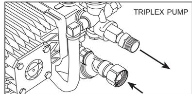
Most pumps are protected by a **thermal valve**. The thermal valve releases water if a pump starts to run too hot. It will prevent catastrophic heat failure. However, the pump may have suffered damage and need maintenance, repair, or replacement. If it does not reset and continues to leak water, the thermal valve may need to be replaced.
