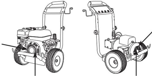
**Pumps are water cooled.** When the machine is running, ensure the trigger of the gun is pressed to allow a constant flow of fresh water into and out of the pump. **Do not let the machine run for more than 30 seconds without pressing down on the trigger.**
