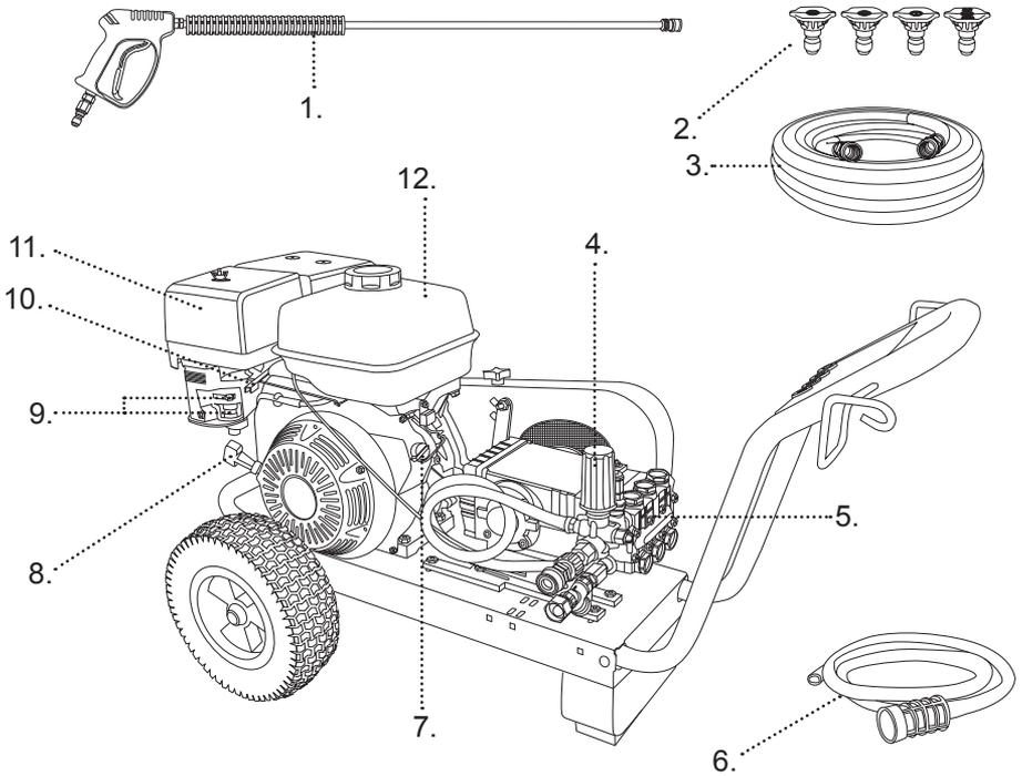
1. **Spray Gun** Controls the application of water onto cleaning surface with trigger device. Includes trigger lock. Allows you to switch between various spray tips.
