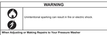
• Disconnect the spark plug wire from the spark plug and place the wire where it cannot contact spark plug.
